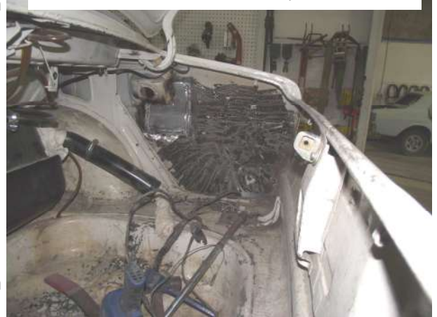
Datto Two—Collision and rust repair RH Rear
