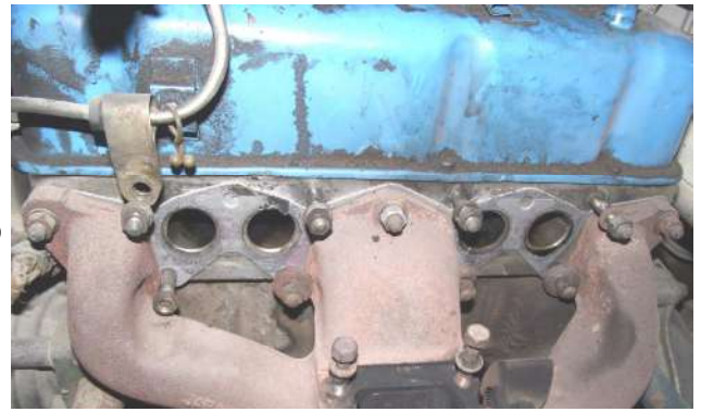
Inlet manifold bolt pattern on the A12A. You can see the small dimple marks where the bolts would normally go for a “normal” manifold.
