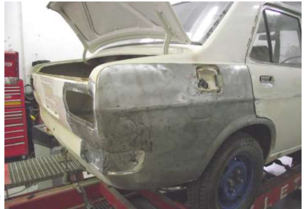
Datto Two—Collision and rust repair RH Rear
