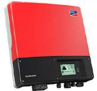
A "grid tie" solar inverter synchronises with the 50Hz AC power network and then converts the DC from solar cells or batteries to AC.
