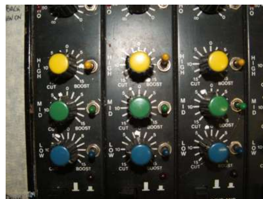
Photo : Close up of the Jands 26/4/2 EQ. The switches (obviously an early modification in the mid '70s) sweep each EQ filter either up or down by about one octave to create a crude but very musical parametric EQ, unique to this design.
