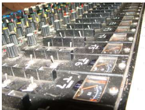
Photo : Jands 26/4/2 with last 8 inputs reconfigured for recording returns From the Tascam 88 1/2” 8 Track.
